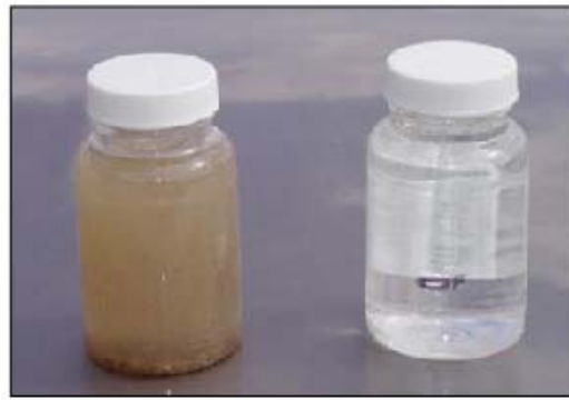
Fig. 1 - Residential wetland wastewater treatment system Fig. 2 - Septic tank effluent (left) vs. wetland effluent (right)
